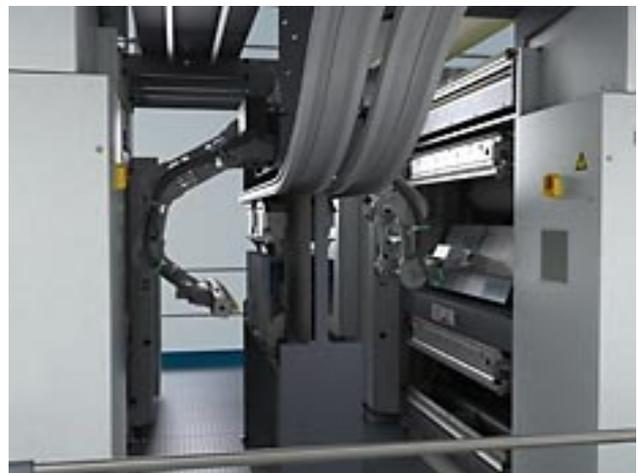
*The system enables an almost fully automatic plate change process – with APL logistics only the disk storage must be loaded manually by the operator in the sound insulated room.*
